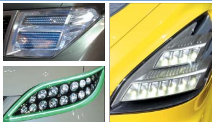
Fig. 4. The lower output power of LEDs dictates a multi-element headlamp design. Credit: Fausto Bigi and Jean-Paul Charret, Valeo Signals and Lighting.
