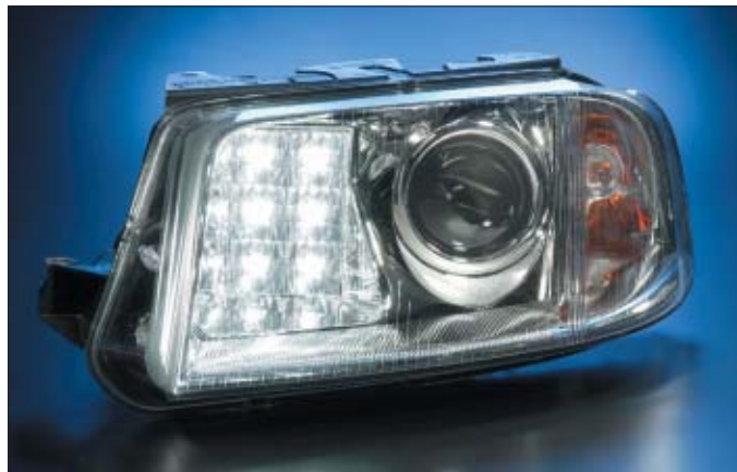
Fig. 5. LED and HID lamps complement each other in this headlight (left) and daytime running light (right) fixture. The configuration was designed and manufactured by Hella and is installed in the Audi A8 sedan. Credit: Karsten Eichhorn, Hella.
